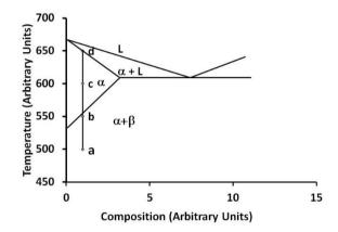
At which temperature will a sample get solutionized the fastest?
