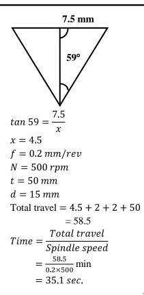
35. Details pertaining to an orthogonal metal cutting process are given below.
