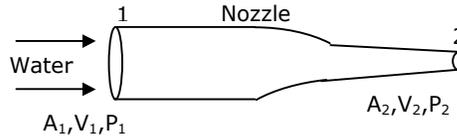
At inlet:  $A_1 = 10^{-3} \text{ m}^2$ ;  $V_1 = 2 \text{ m/sec}$ ;  $P_1 = 3 \times 10^5 \text{ Pa (gauge)}$
