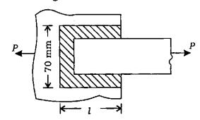
The maximum tensile and shear stresses are 70 N/mm<sup>2</sup> and 56 N/mm<sup>2</sup> respectively. The plate is 70 mm wide and 12.5 mm thick. What will be the value of l if the total load carried by the joint is 85 kN?
