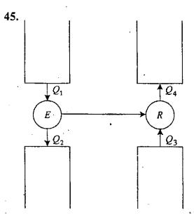
In the figure shown above, E is the heat engine with efficiency of 0.4 and R is the refrigerator. If  $Q_2 + Q_4 = 3Q_1$ , the COP of the refrigerator will be
