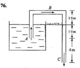
A tube is used (as shown in the above figure) as a siphon to discharge an oil of specific gravity 0.8 from a large open vessel into a drain at atmospheric pressure. The velocity of oil through the siphon will be
