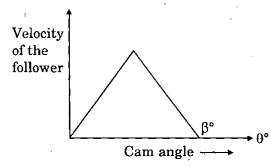
The above figure shows the required velocity profile for a follower of a cam during its rise. If the driving cam is rotating at a uniform velocity, the nature of displacement recommended for the follower is
