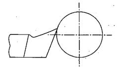
The effect of centering error when the tool is set above the center line as shown in the figure results effectively in
