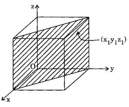
Miller indices (x, y, z) for the hatched plane in the above unit cell are represented as
