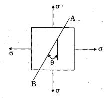
A point in two-dimensional stress state, is subjected to biaxial stress as shown in the above figure. The shear stress acting on the plane AB is
