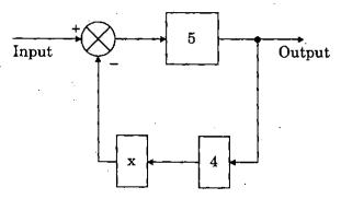
The above figure shows the block diagram of an automatic control system having bounded input. The output becomes unbounded if the value of x is
