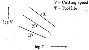
The above figure shows a typical relationship between tool life and cutting speed for different materials. Match the graphs for HSS, Carbide and Ceramic tool materials and select the correct answer using the code given below the lists:
