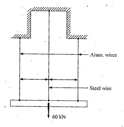
If a load of 60 kN is applied to a rigid bar suspended by 3 wires as shown in the above figure what force will be resisted by each wire?
