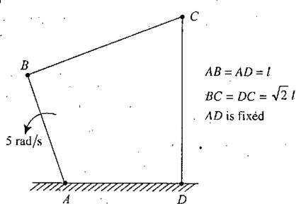
The driver link AB of a four bar mechanism is rotated at 5.0 rad/s in counter clockwise direction as shown in the above figure. Locate and indicate the Instantaneous Centre (I.C.) of the coupler BC with respect to fixed link AD at an instant when  $\angle BAD = 180^{\circ}$ . Find angular velocity of the coupler using 1.C. method only.
