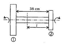
The above figure shows two rotors connected by an elastic shaft undergoing torsional vibration. The rotor ① has a mass of 2 kg and a diameter of 60 cm, while the rotor ② has a mass of 1 kg and a diameter of 20 cm. What is the distance l at which the node of vibration of torsional vibration occurs?
