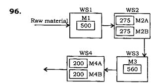
A product is manufactured by processing on the four workstations (WS). The capacity of each machine on these work-stations is given in the diagram as shown above. In the diagram M1, M2A, M2B, M3, M4A and M4B are the machines and 500, 275, 275, 560, 200 and 200 are their capacities in number of products made per shift. If the products made in this system are 5% defective, then what will be the output from this system?
